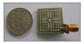
Fig. 2 Fabricated prototype of the proposed antenna
